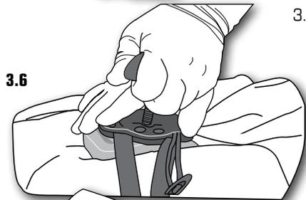
3.6 With one hand on the base plate, grip the threaded T-handle and rotate it clockwise to tighten
