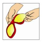
Working from the front of the goggles, insert the upper corner of the lens into corresponding eyepiece starting closest to the nose area. Make sure the keyhole retention notch in the upper corner of the lens is aligned and securely fitted onto the appropriate post within the eyepiece gasket.
